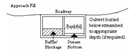
(7) Where adjacent floodplain is available, flows exceeding bankfull will be accommodated by installing culverts/pipes at the floodplain elevation. When multiple culverts/pipes are used, baseflow must be maintained at the appropriate width and depth by the construction of floodplain benches, sills, and/or construction methods to ensure that the overflow culvert(s)/pipe(s) is elevated above the baseflow culvert(s)/pipe(s).
